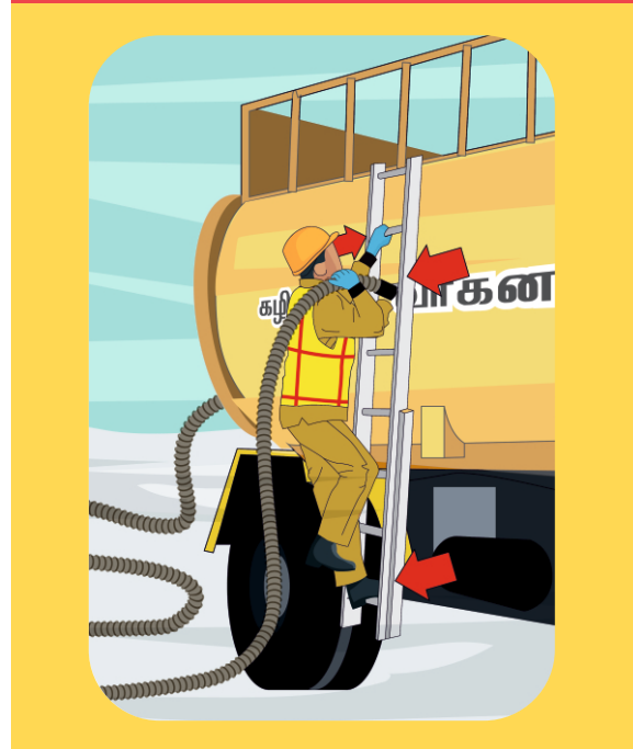
Figure 25: Mounting Hose on De-sludging Truck
