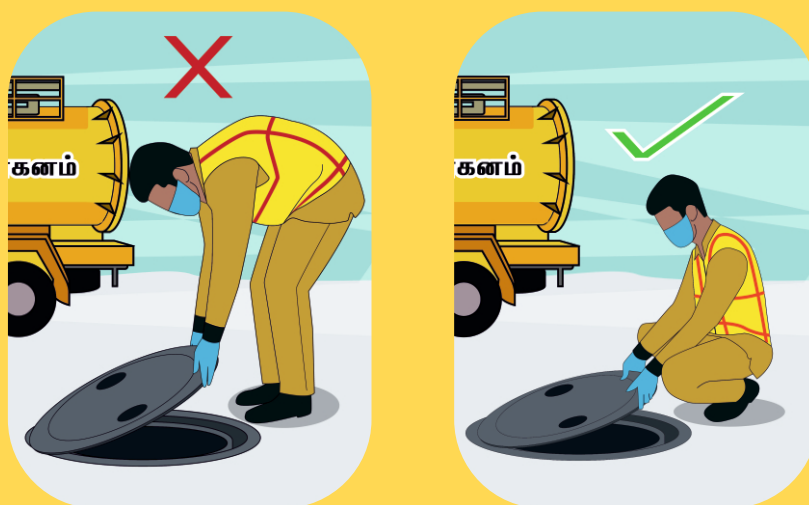
Figure 28: Right Posture to Open a Septic Tank
